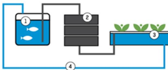
Fig. 1: Simplified schematic diagram of an aquaponic system (Leskovec, 2013)
