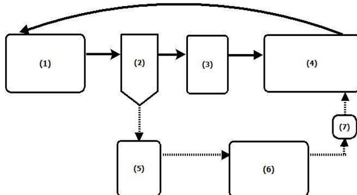
Fig. 2: Schematic diagram of the pilot integrated system: (1) fish tank; (2) sedimentation for solids collection; (3) biofiltration; (4) hydroponic DWC; (5) off-line mineralization; (6) *Spirulina* cultivation; (7) foliar application of *Spirulina* (Hartman, 2015)
